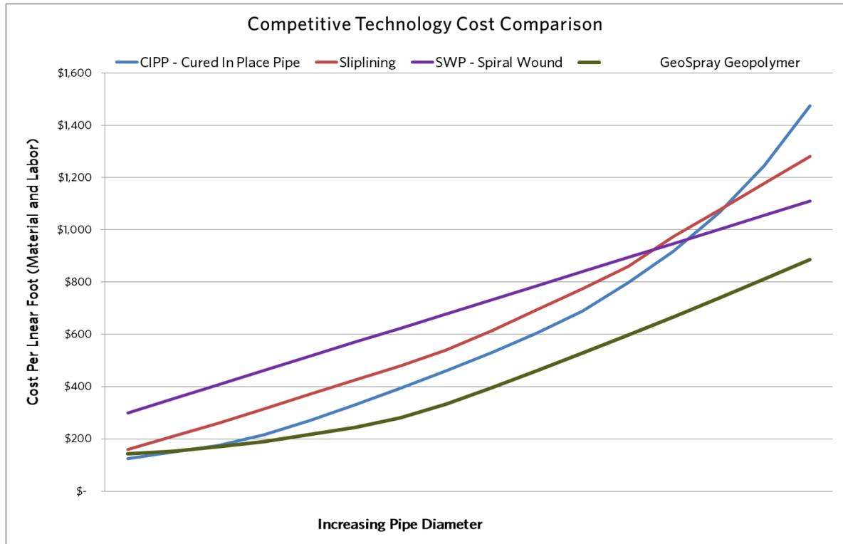
Figure 5: Cost comparison of competitive trenchless technologies
