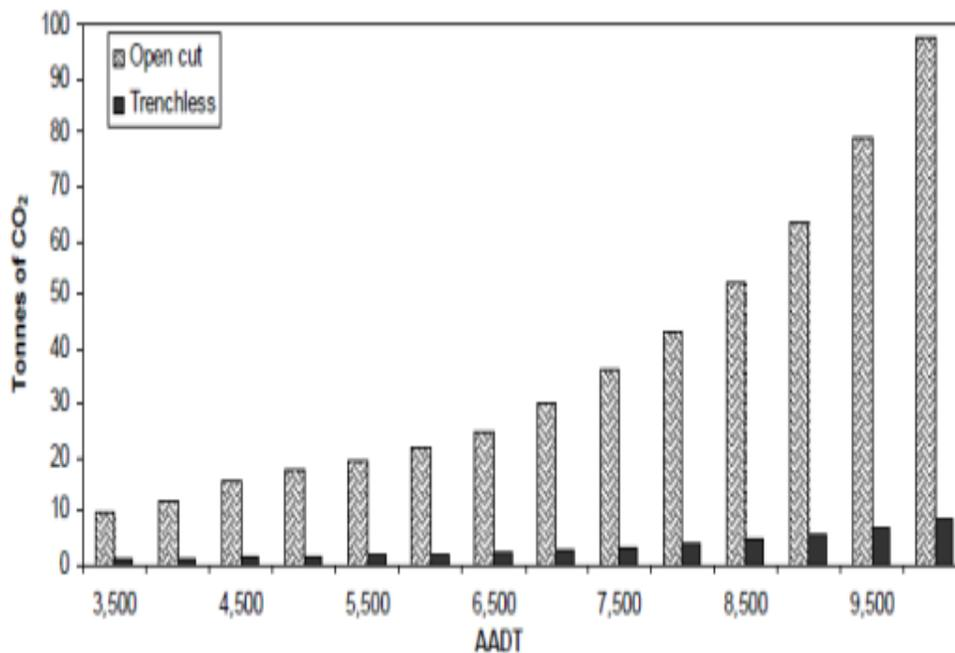
Figure 4: Comparison CO<sub>2</sub> Emissions of traditional open cut versus trenchless pipe repair<sup>10</sup>
