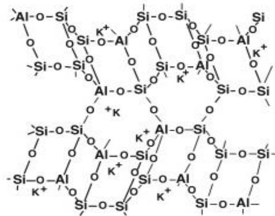
**Figure 1: Example Aluminosilicate Geopolymer Structure<sup>7</sup>**
